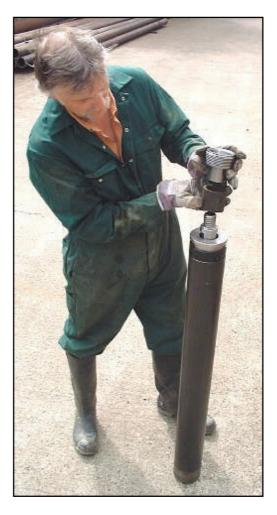
33. Drive the Casing + Sampler fully into the ground until the casing drive head is positioned in the middle of the slip bowl. Attach the casing spanner to the slip bowl.
