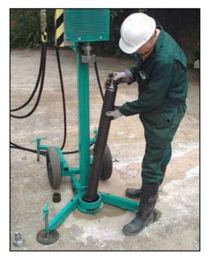
23. Attach the sample tube to the drill rig using the bottom adaptor shown here.
