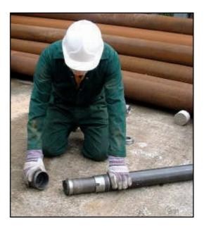
25. To extend the depth of the sample use the extension rods provided. The first rod used must be the STARTER ROD which is 60 mm shorter than the standard rods.
