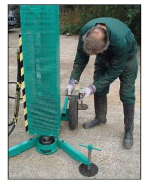
6. Apply grease to the slide before each use of the rig. This increases the life of the brass slides on the weight.
