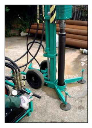
40. To extract the sampler uncouple the drill rods, each time securing the rod with the rod spanner placed over the slip bowl
