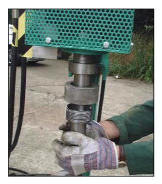
24. Drive the sample tube fully into the ground by operating the chain motor (Right-hand lever). Then operate the hydraulic cylinder (Left-hand lever) to extract the tube. Detach the sample tube from the rig and extract the plastic liner containing soil sample.
