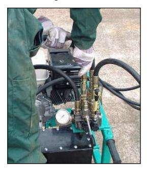
8. The snap-on couplings enable the hoses to be coupled and uncoupled quickly.
