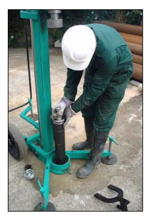
37. Attach another length of casing and the STARTER ROD to the top of the sampler.
