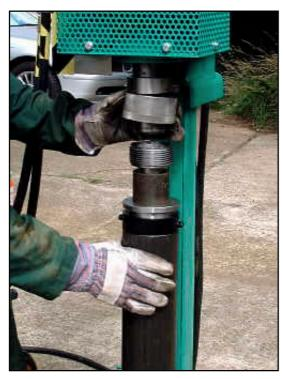
31. Place the Drive Ring into the top of the casing, add the spacer tube and screw the bottom adaptor onto the top of the sample tube
