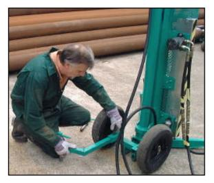
4. Level the rig by screwing the feet onto the load bearing plates. The mast must be vertical for correct operation. Tools may become stuck in borehole if mast is inclined at an angle.
