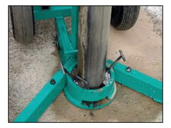
43. It is possible to sample the ground below the level of the installed casing by reducing the size of the sampler from 101 mm to 92 mm or smaller.
