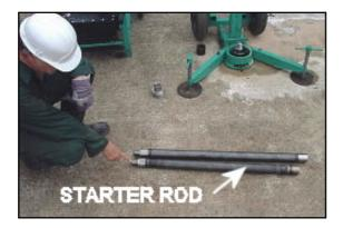
26. Drop the empty sample tube down the hole and attach the rod to the top of the sampler tube, with the male thread facing upwards.
