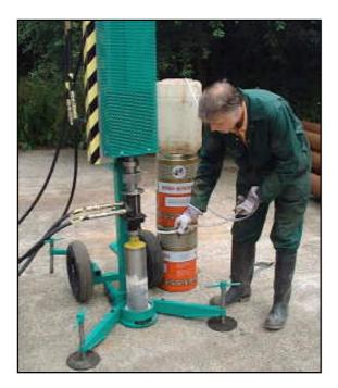
16. Siphon the water from the container through a hose and attach this to the hose spigot on the Coring Unit. The flush must be maintained continuously when coring.
