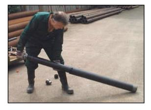
32. Fit the casing and sampler to the rig using the bottom adaptor as usual.
