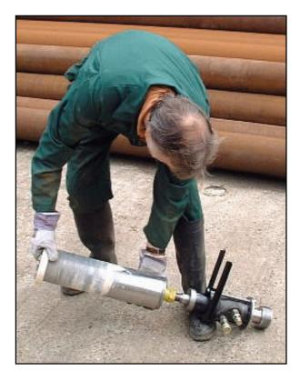
14. Attach the Coring Unit onto the rig at the base of the anvil. Connect the hydraulic hoses leading from the Right-Hand side of the control block onto the snap-on couplings of the Coring Unit. (these hoses may first need to be disconnected from the chain motor).
