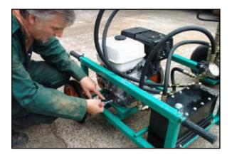
10. Check Hydraulic Oil Level before starting the engine.
