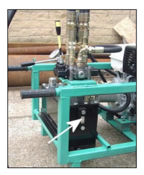
11. Start the engine following the instructions in the separate Engine Manual and raise the Carriage to its uppermost position using the Left-hand lever on the Control Block.
