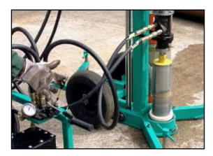
18. Lower the carriage fully using the Lefthand lever on the control block so that its weight is bearing down fully on the core bit. Ensure that the nylon ring is in place on the core bit to stabilize the bit in the slip bowl. Adjust the speed of the engine until you obtain maximum rate of penetration.
