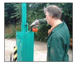
7. Connect the hydraulic hoses. The pair hoses from the left hand side of the control block connect to the hydraulic cylinder. The pair of hoses from the righthand side connect to the chain motor (or concrete coring attachment when in use)
