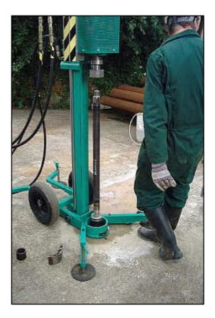
27. Attach the rod to the rig using the same adaptor as before.
