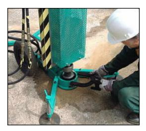
34. Use the hydraulic cylinder to extract the sampler. The casing stays in place in the ground.
