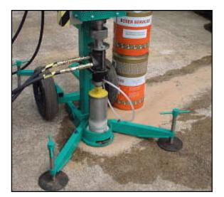
20. After cutting through the concrete raise the carriage slowly and then stop the bit rotating. Remove the concrete core and detach the Coring unit from the rig.
