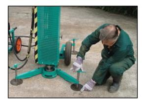
5. Remove the safety pin from the slide to enable the weight to slide freely.(Remember to replace this when transporting the rig)
