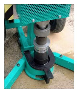
35. After extracting the sample tube, remove the sample from the tube and replace with a new plastic liner.
